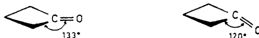
Figure 5.5 Without quadratic terms, the exocyclic atom would move exaggeratedly out of plane to restore a 120^\circ valence angle.
