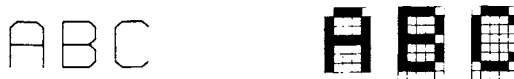
Figure 1.12 Generation of a character from vectors or pixels of a dot matrix.
